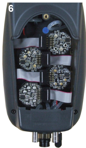
Connection of the sensor ribbon cable
